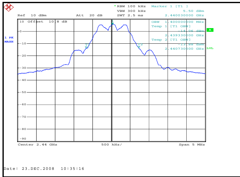
Figure 7.4.2-5: 99% Bandwidth Plot – Mid Channel
