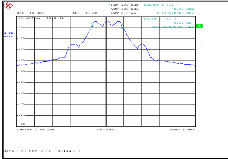
Figure 7.4.2-2: 6dB Bandwidth Plot – Mid Channel
