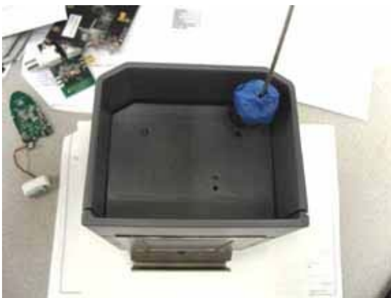
Figure 3 Ferrite decoupling bead on coax, bottom view of RSI-290 case.
