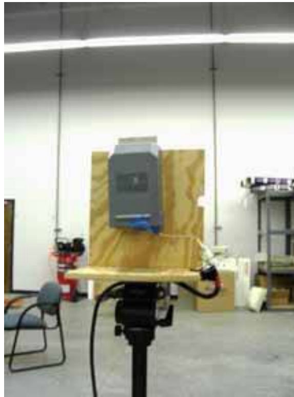
Figure 4. Mounting for azimuth measurements
