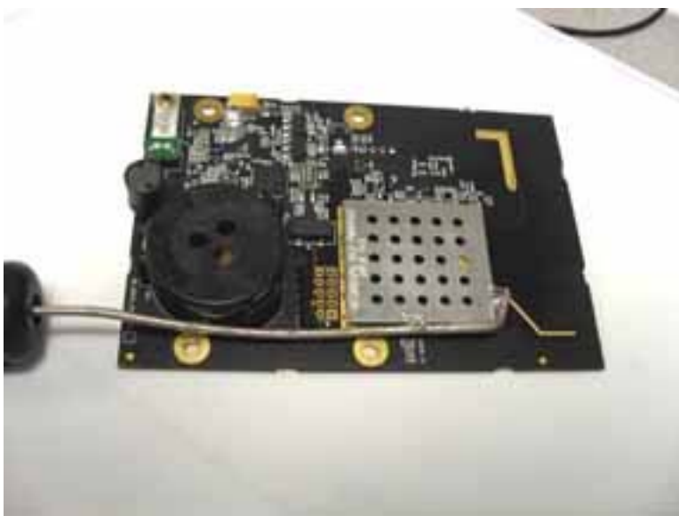
Figure 2 Attachment of semi-rigid coax to board and antenna, prior to mounting in RSI-290 case.
