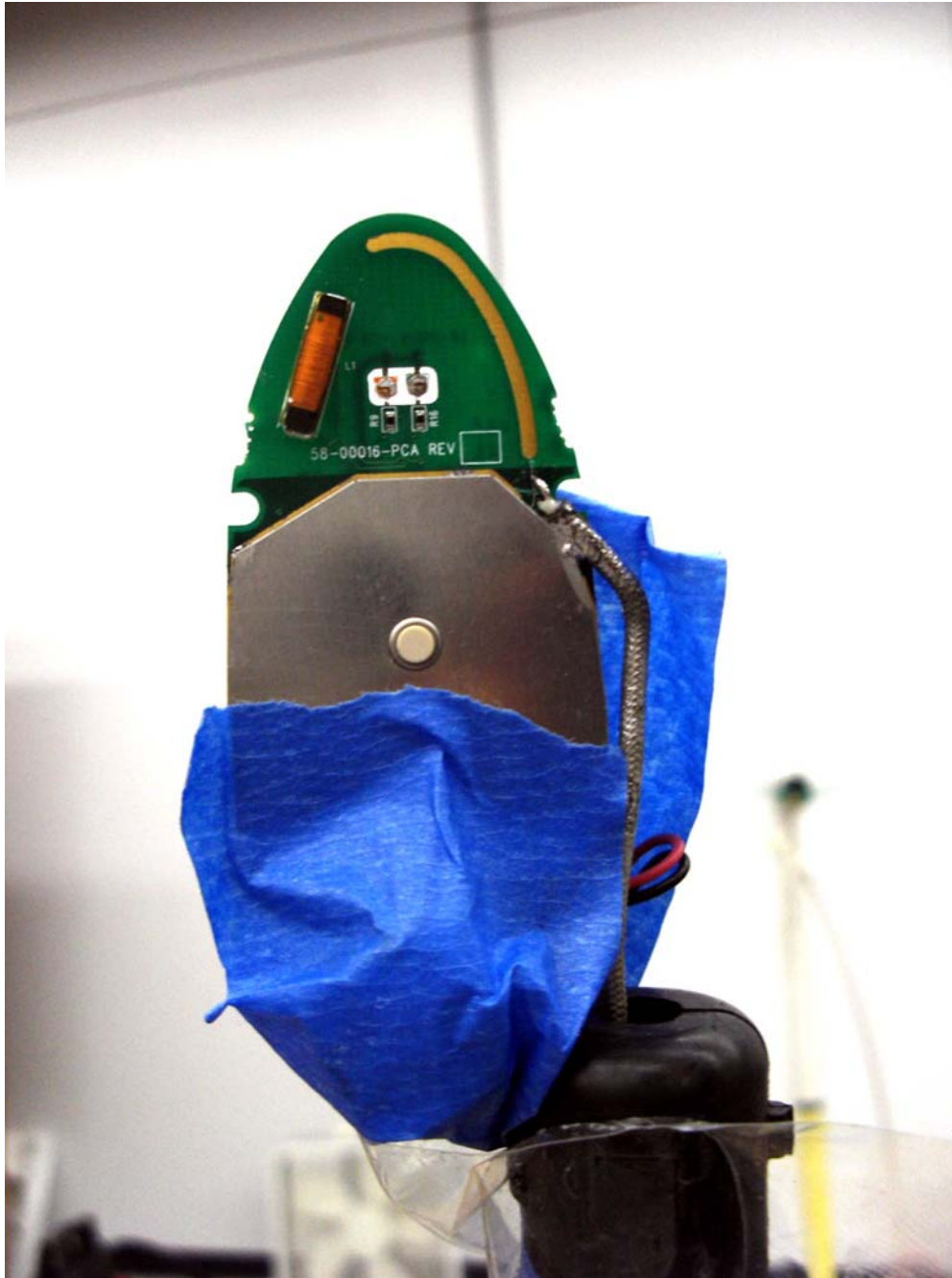
Figure 3. Test Setup for Azimuth Measurement
