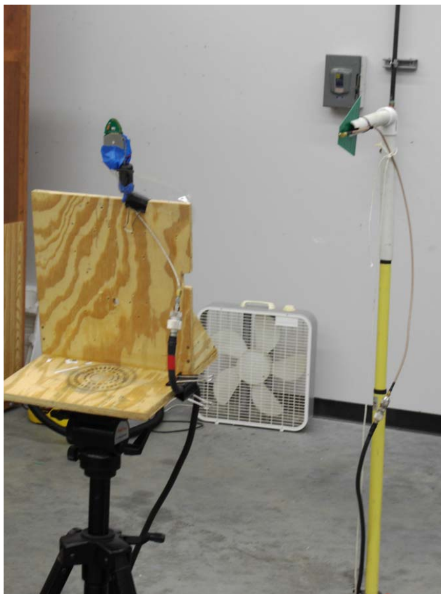
Figure 2 Log-periodic (source) and test antenna. System path loss was calibrated with a reference dipole prior to DUT measurement.
