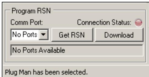
4. Under **Comm Port**, click the drop-down list and select the correct Comm Port for use with this device.
