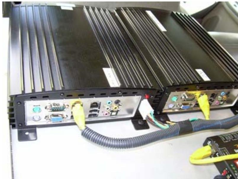
**Figure 9: MMR System and Gateway Server**
