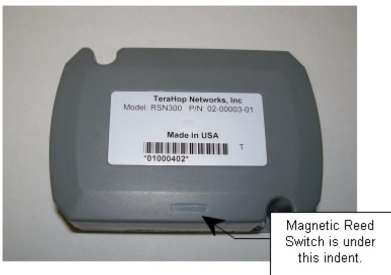
**Figure 16: Magnetic Reed Switch Indent on RSN**
