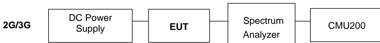
Fig. 2-1 Configuration of Tested System (Fixed Channel-Conducted)
