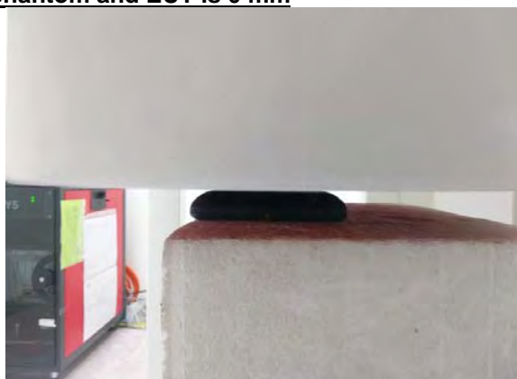
Fig.3 EUT Back side to flat phantom
