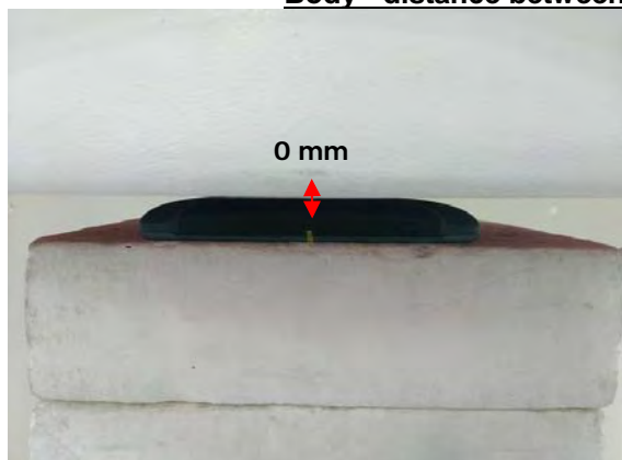
Fig.3 EUT Back side to flat phantom
