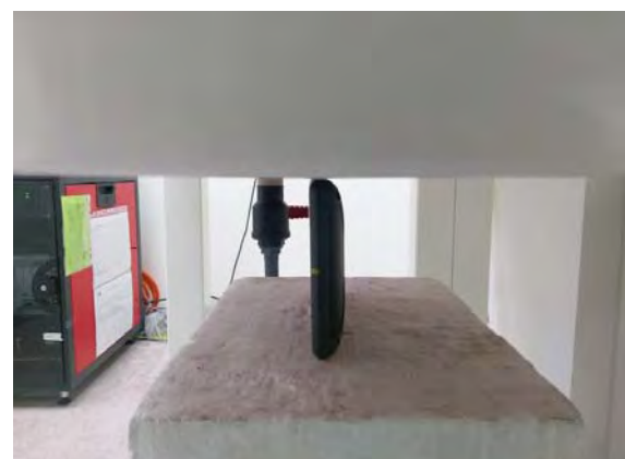
Fig.4 EUT Top side to flat phantom
