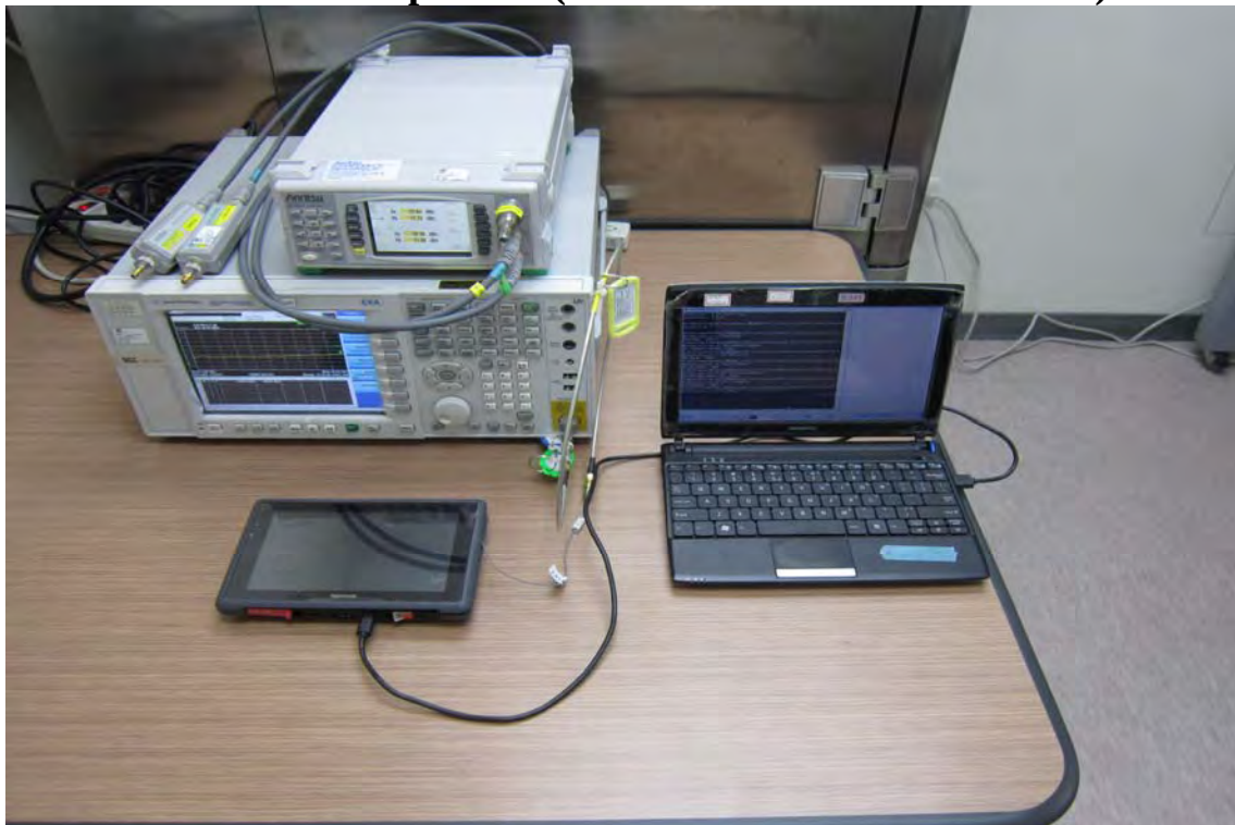
Conducted Setup Photo (Measurement at Antenna Port)
