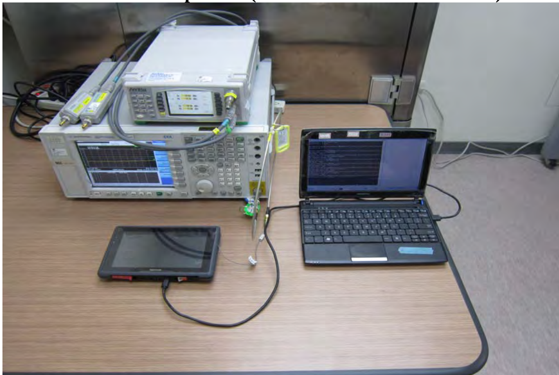
Conducted Setup Photo (Measurement at Antenna Port)
