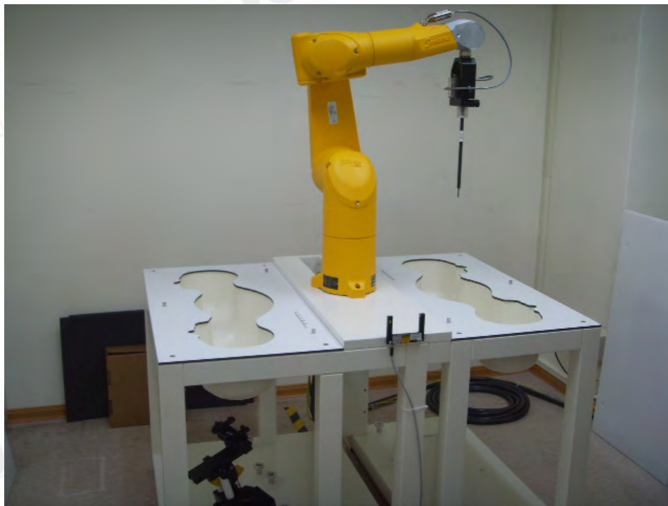
Fig.1 Photograph of the SAR measurement System
