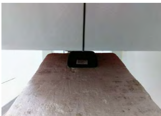
Fig.8 EUT Back side_curve (0mm) to flat phantom
