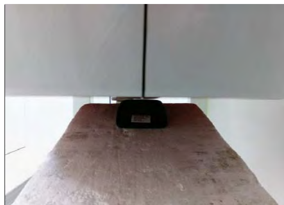
Fig.7 EUT Back side_curve (1mm) to flat phantom
