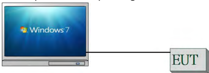
Fig 2-2 Conducted (AC power line) Configuration
