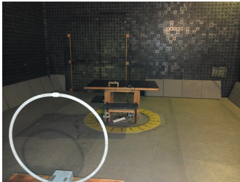
Photograph 7.1.1 Setup for spurious emission field strength measurements below 30 MHz
