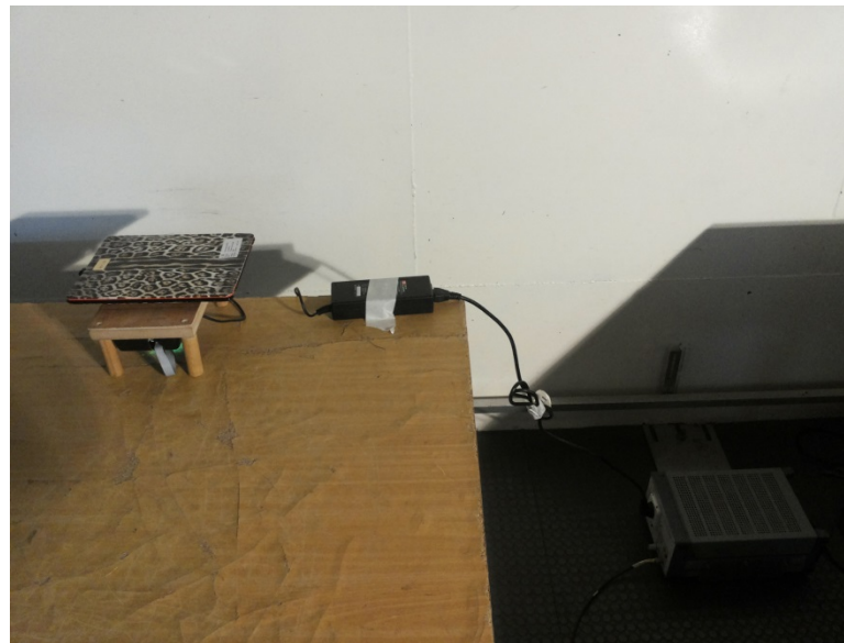
Photograph 7.2.1 Setup for conducted emission measurements, PMA 15 Watt mode
