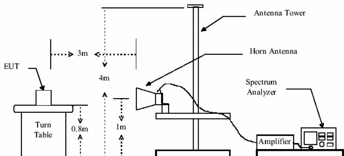
The field strength is calculated by adding the Antenna Factor, Cable Factor & Peramplifier . The basic equation with a sample calculation is as follows:
