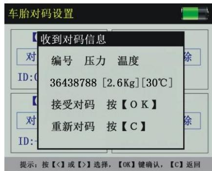
Select **【OK】**, the system will be numbered from 36438788 transmitters in the host, the next received signal will be updated as the transmitter information, and displayed on the home page.
