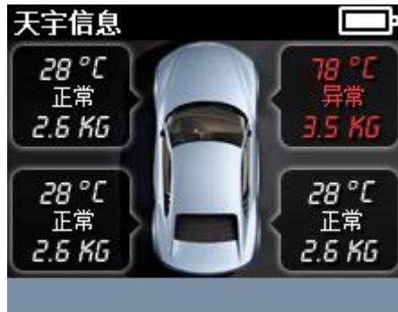
If a tire temperature or pressure anomaly, backlight will automatically light up, screen corresponding to the position in red font, while displaying the " abnormal tyre pressure or temperature anomalies, " buzz reminds, the user can press the **【OK】** or **【C】** button to turn off the alarm, otherwise the main machine will be every 30 seconds alarm 1 second, each with a 1Hz frequency buzzer by 8 times.
