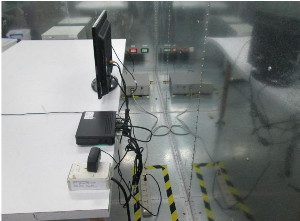
**Radiated Emission Below 1GHz Test**
