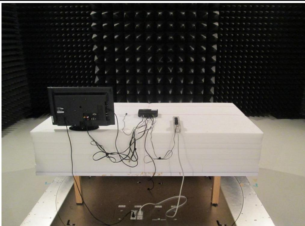
**Radiated Emission Above 1GHz Test**
