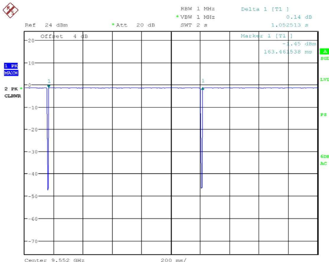
The Pulse Width measured was 1.03648 seconds.
