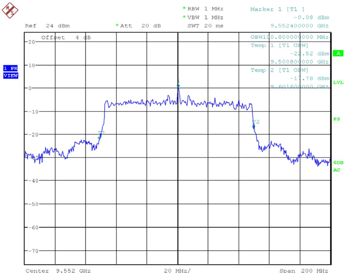
The occupied bandwidth (OBW) was measured to be 100.8 MHz.
