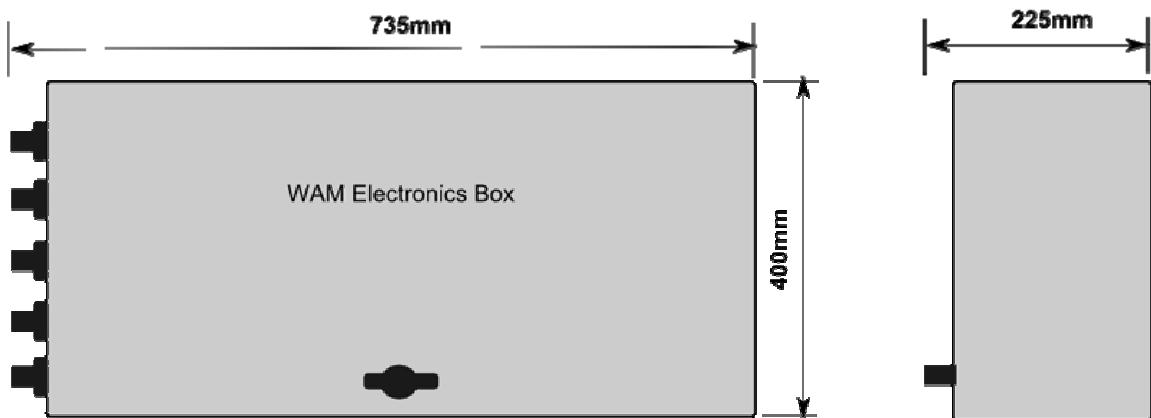
The Work Area Monitor (WAM) is used by open-pit mines as a safety device to monitor the movements of mine walls and provides notification alerts when detected wall movements.
