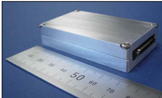
When GSM communications are unavailable, data is logged to non-volatile flash memory for sending when communications resume (or downloading over GPRS upon request). The WP0100NS has sufficient on-board flash memory for storage of 10,000 individual position/time/date/status reports.
