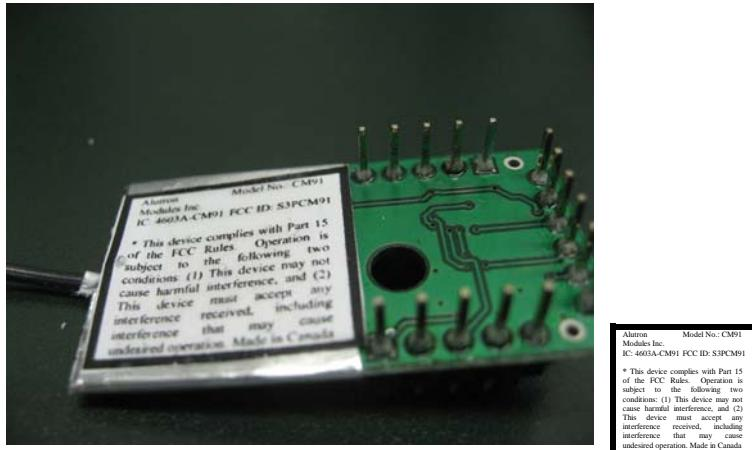
This label is in full scale. Its dimensions are 2cmx2cm. The label is printed on silver paper for easy application and it is permanently affixed.
