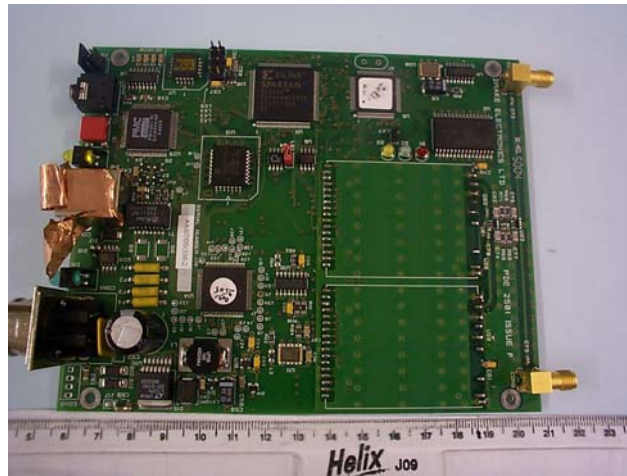
PHOTOGRAPH No. 7 MAIN PCB COMPONENT SIDE RF MODULE REMOVED
