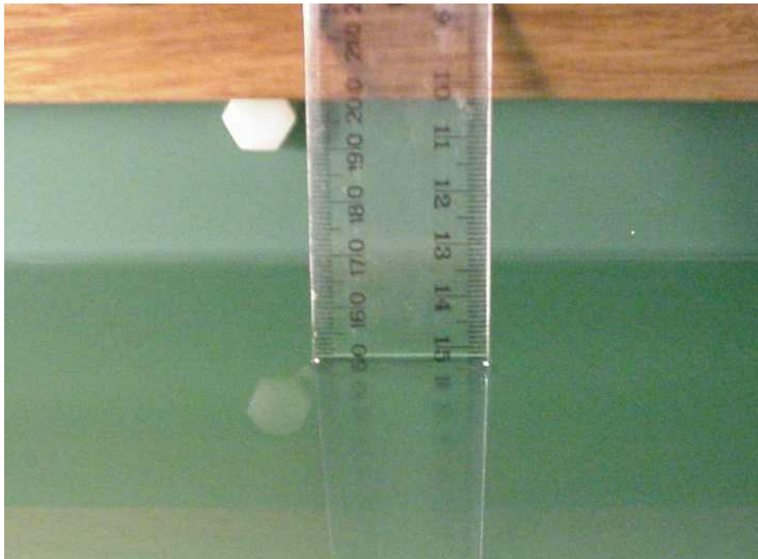
Photo of liquid Depth in Flat Phantom
