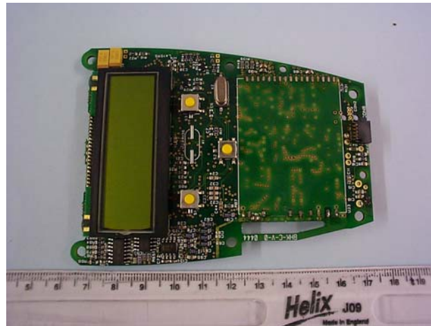
PHOTOGRAPH No. 7 MAIN PCB LCD SIDE RF MODULE REMOVED
