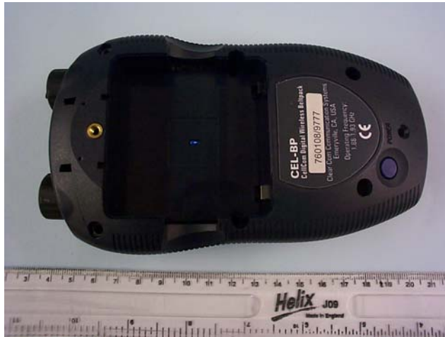
PHOTOGRAPH No. 4 TRANSMITTER REAR VIEW BATTERY REMOVED
