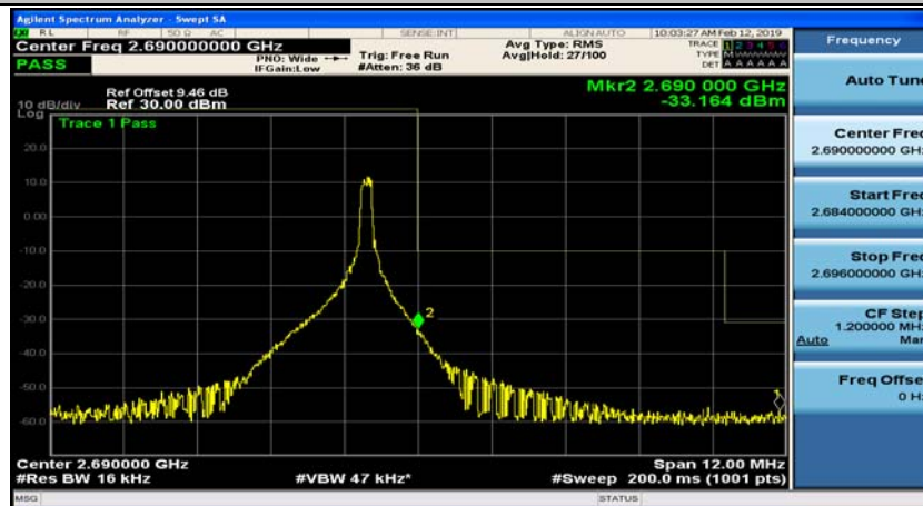
(Channel Bandwidth:15 MHz)_HCH_QPSK_37RB#0
