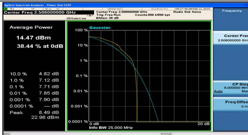
(Channel Bandwidth:20 MHz)_LCH_16QAM_50RB#0
