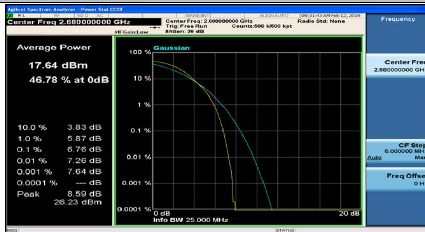
(Channel Bandwidth:20 MHz)_HCH_QPSK_100RB#0
