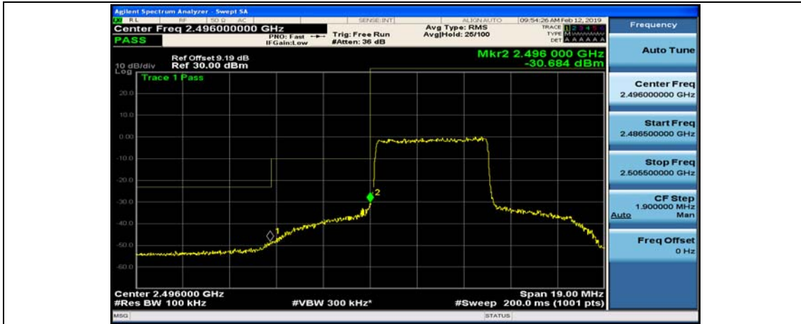
(Channel Bandwidth: 5 MHz)_HCH_QPSK_1RB#0
