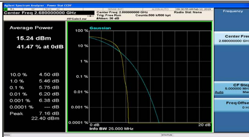
(Channel Bandwidth:20 MHz)_HCH_16QAM_50RB#0
