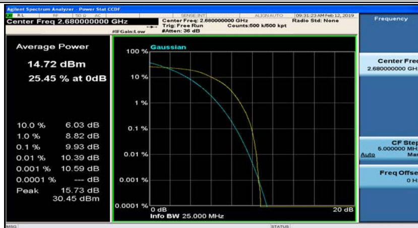
(Channel Bandwidth:20 MHz)_HCH_16QAM_50RB#25
