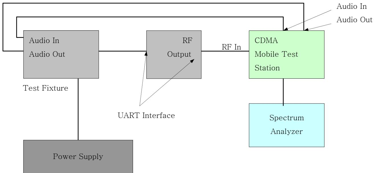
**UART Interface:** The UART Interface has a serial communication link and RF Interface port that can be used to test, debug or upgrade the phone's functions and characteristics.
