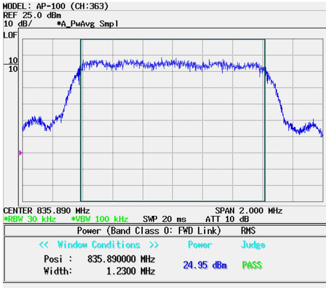
**■ CDMA Mode (0363 CH.) : Occupied Bandwidth**
