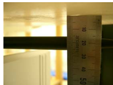
Fig. 21. Body SAR Test Setup with Holster
