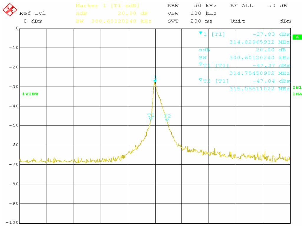
The bandwidth is 300.6KHz which is less than 315MHz \* 0.25% = 787.5KHz.
