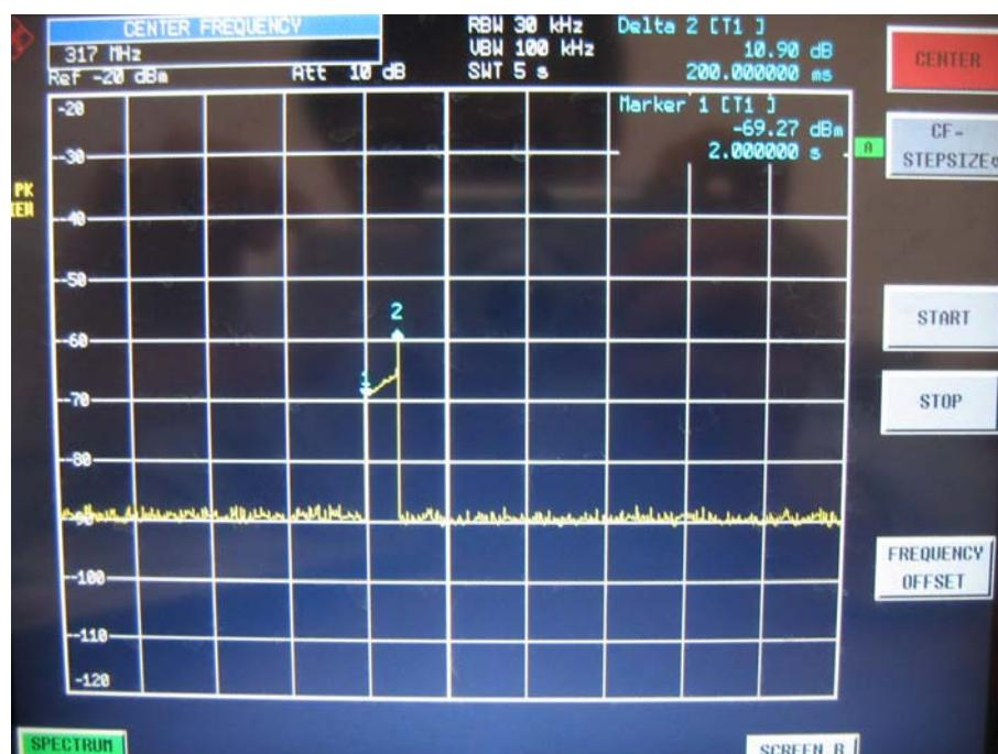
**The results:** The unit does meet the FCC Part 15C Section 15.231 requirements.
