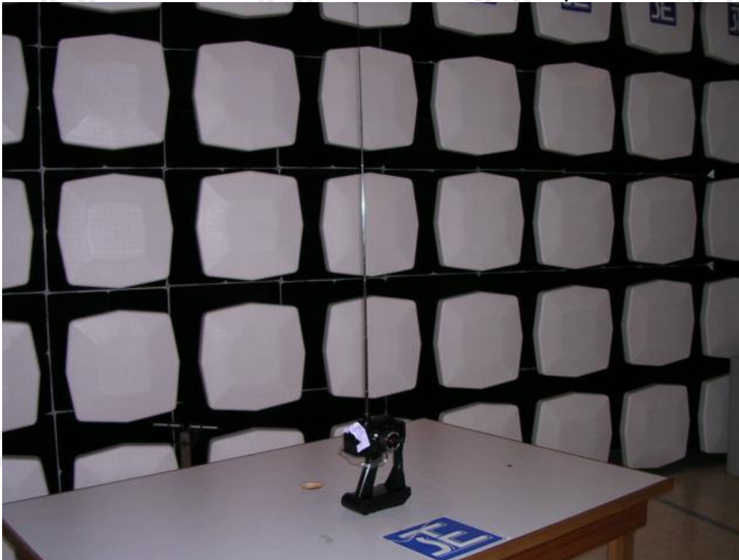
Measurement of Radiated Emission Test Set Up
