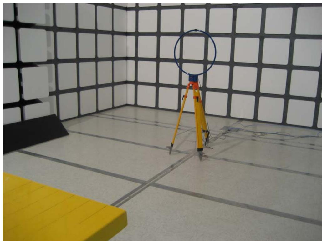
**Test Configuration: 30MHz~1GHz**
