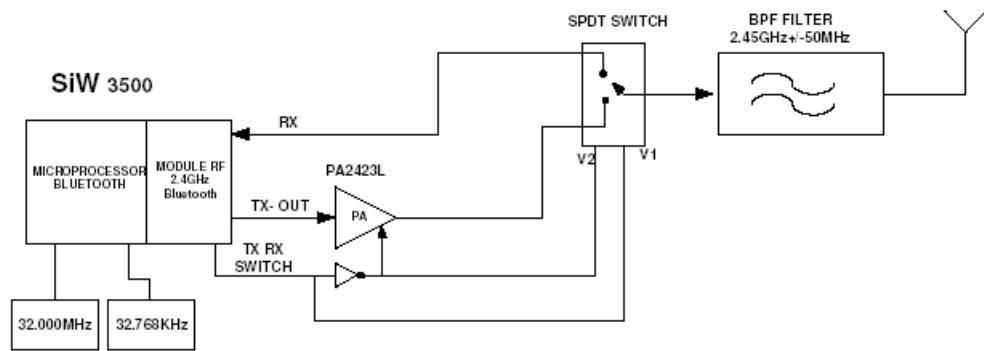
Single -chip IC for Bluetooth wireless technology on chip protocol stack software. The input port [RX] is the normal mode the IC operation and waiting to get order from the master.
