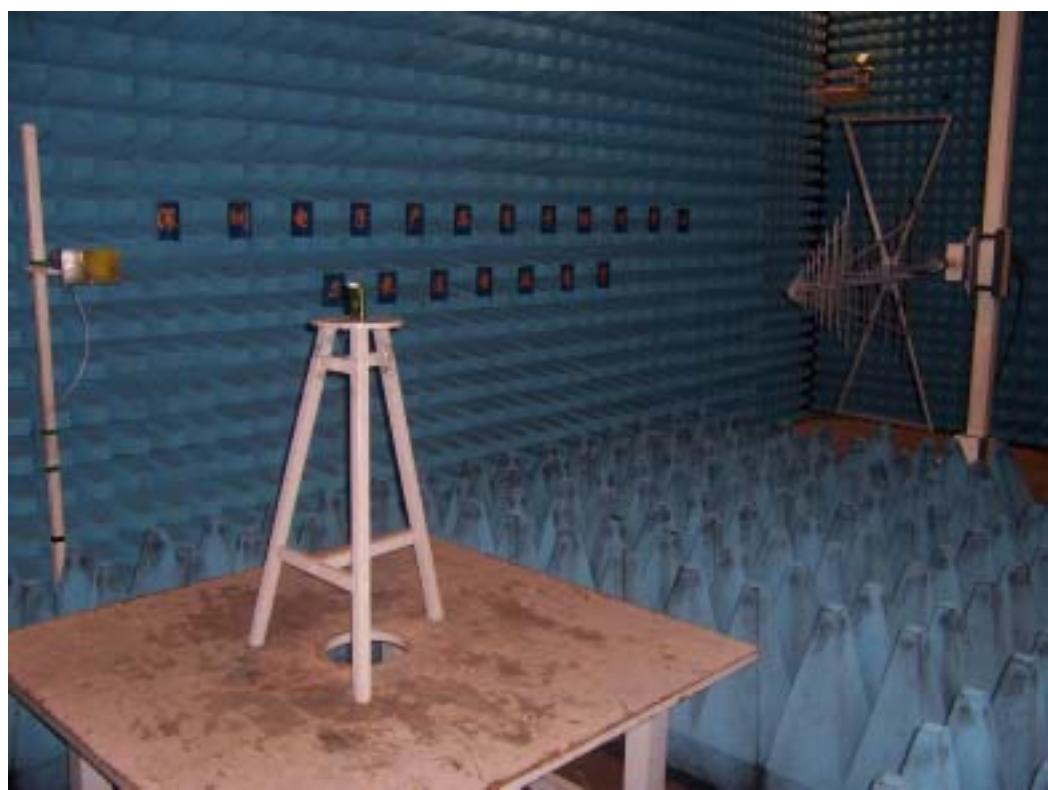
**3. Radiated RF Test (9kHz~30MHz)**
