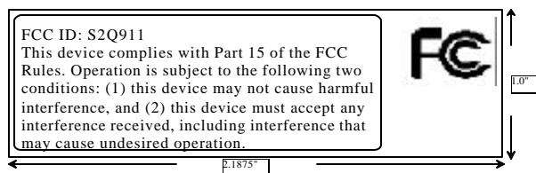
**Specifications:** The bottom sticker is black in color. Text is white in color and is center justified. Labels are printed in indelible ink on permanent adhesive backing and shall be affixed at a conspicuous location on the EUT.
