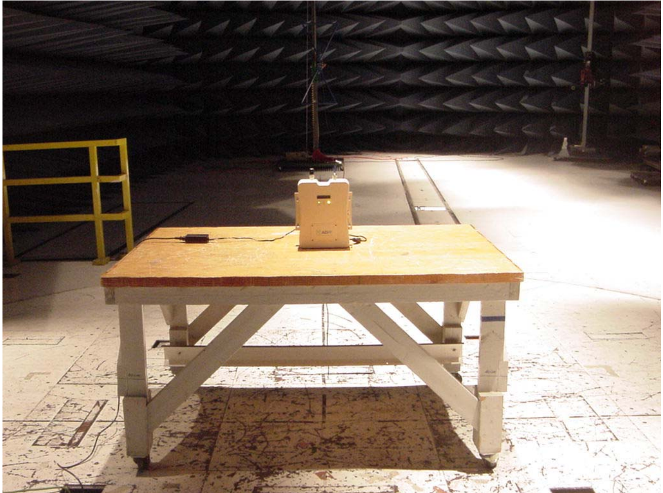
Photograph 3. Radiated Emission Limits Test Setup
