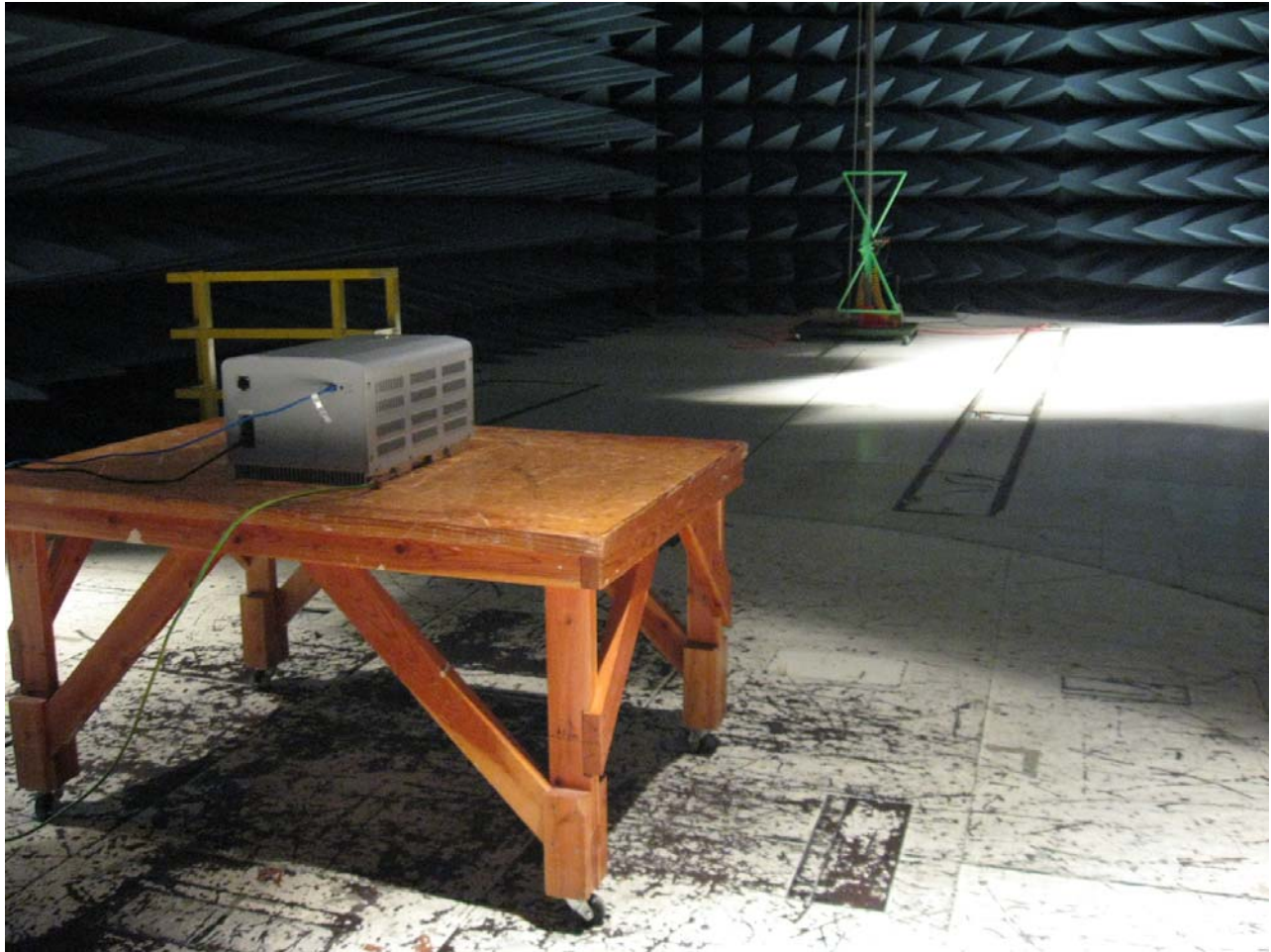
Photograph 3. Radiated Emission Limits, Test Setup
