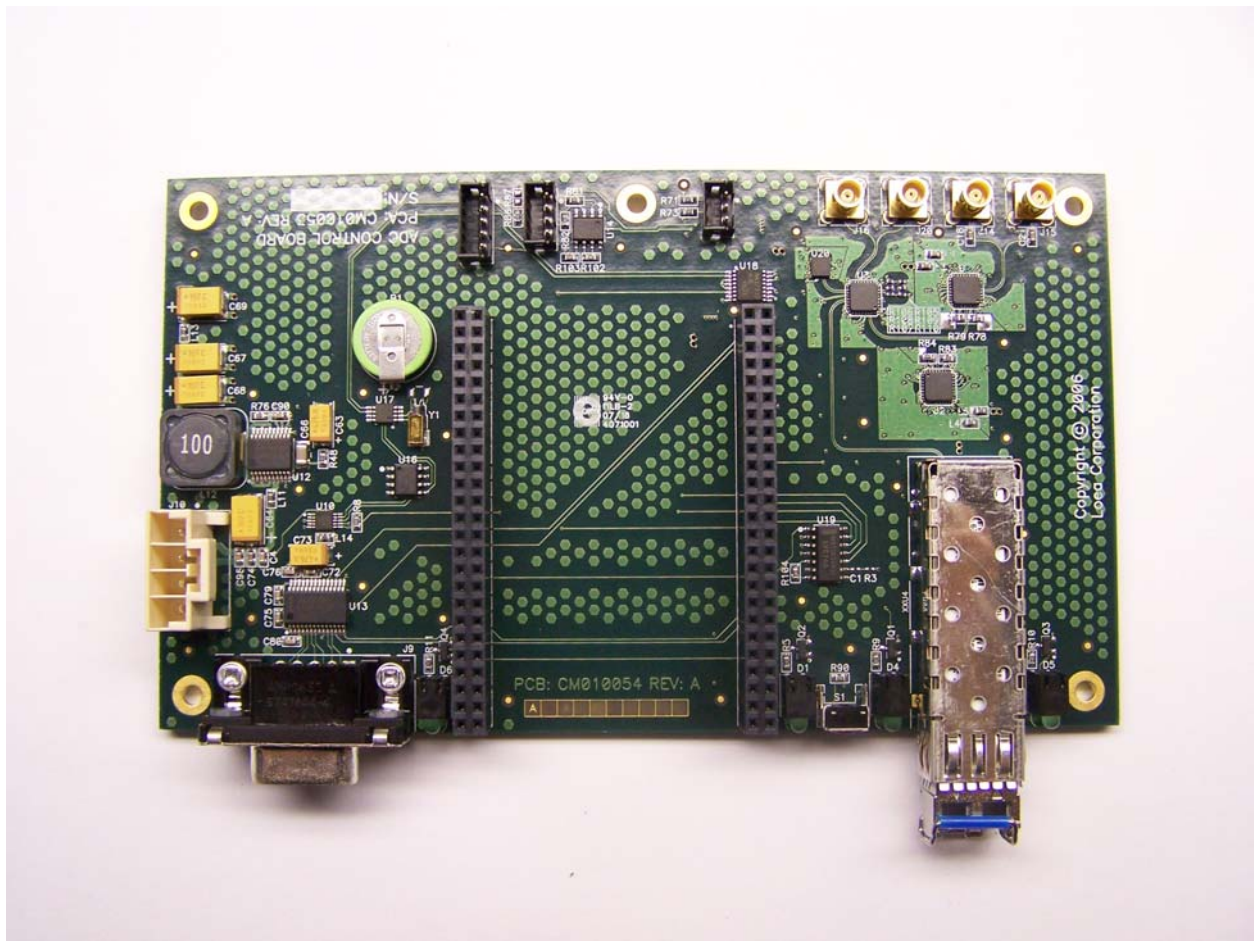
Photo of Control board – Top view with Netburner board removed
