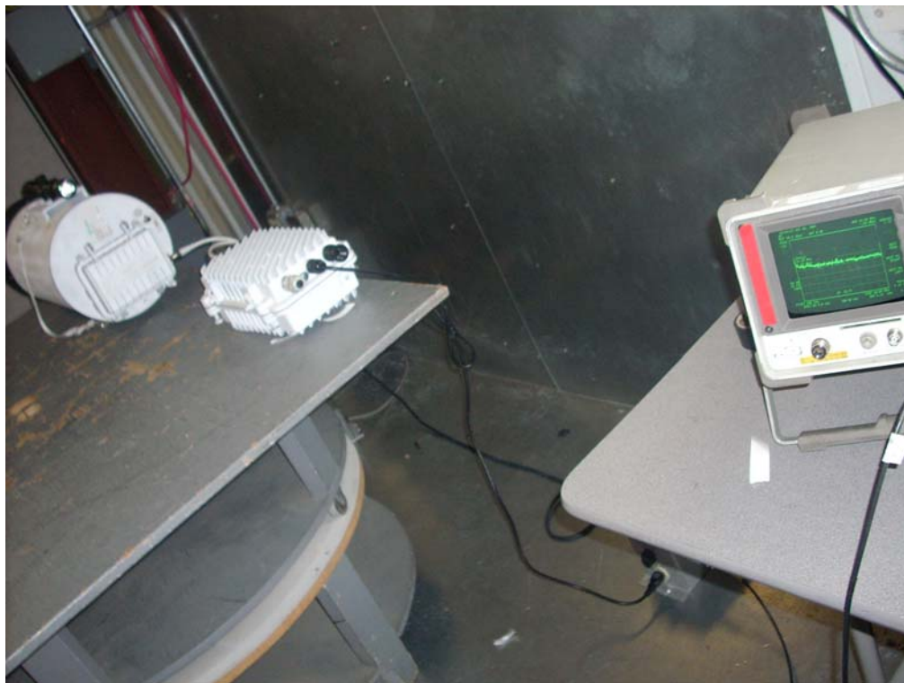
AC Mains Conducted Emission – Front
