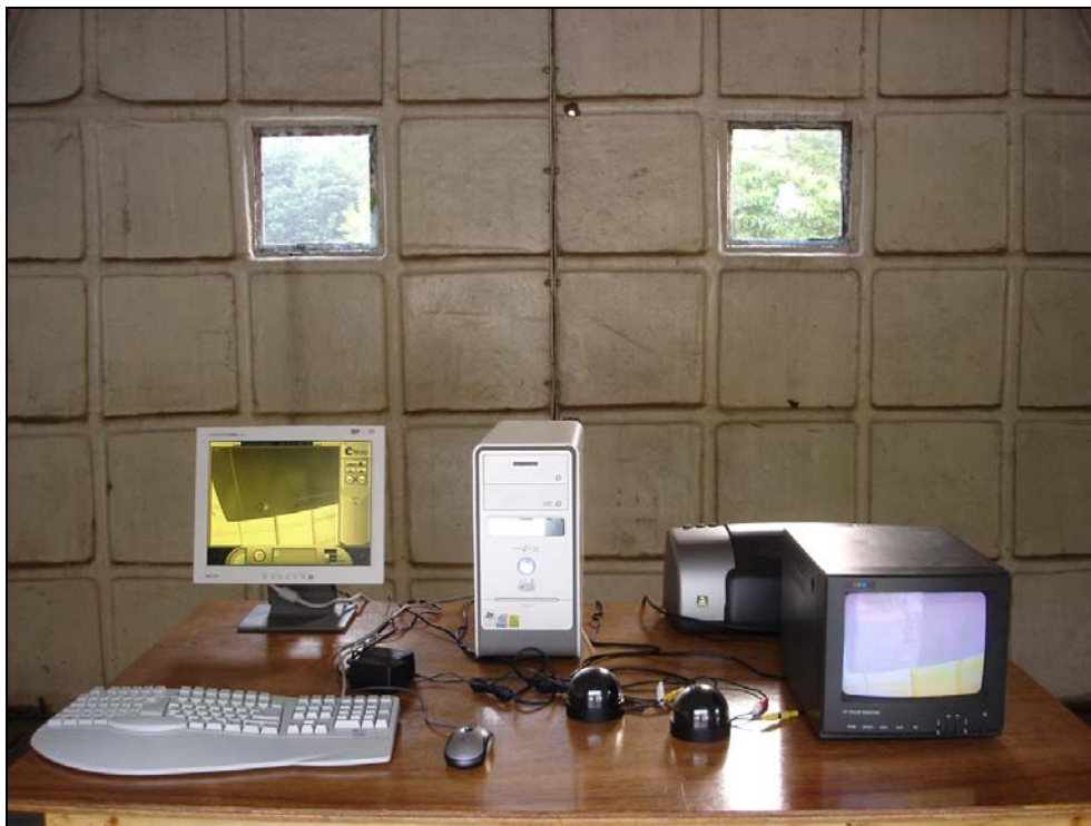
Photograph 2: Setup for Radiated Emissions
