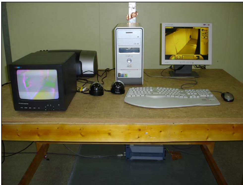
Photograph 1: Setup for Conducted Emissions
