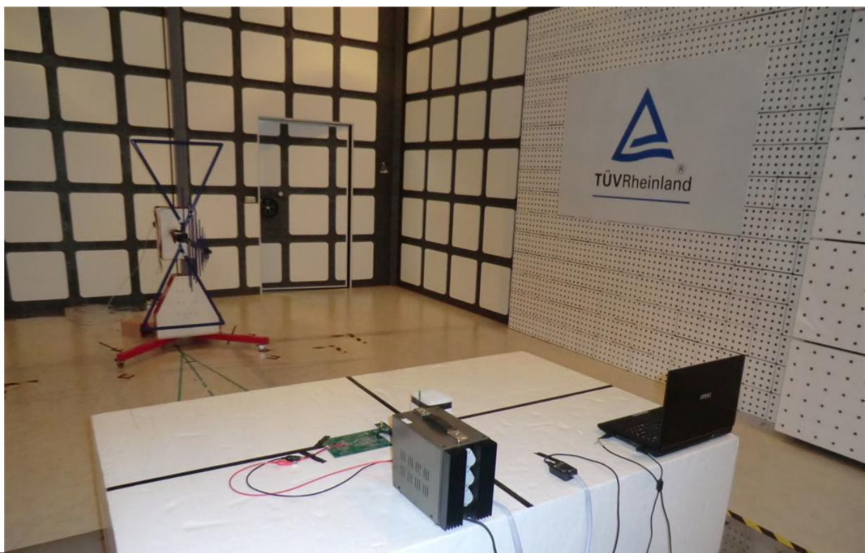
Photograph 2: Set-up for Spurious Emissions (Back View 1)
