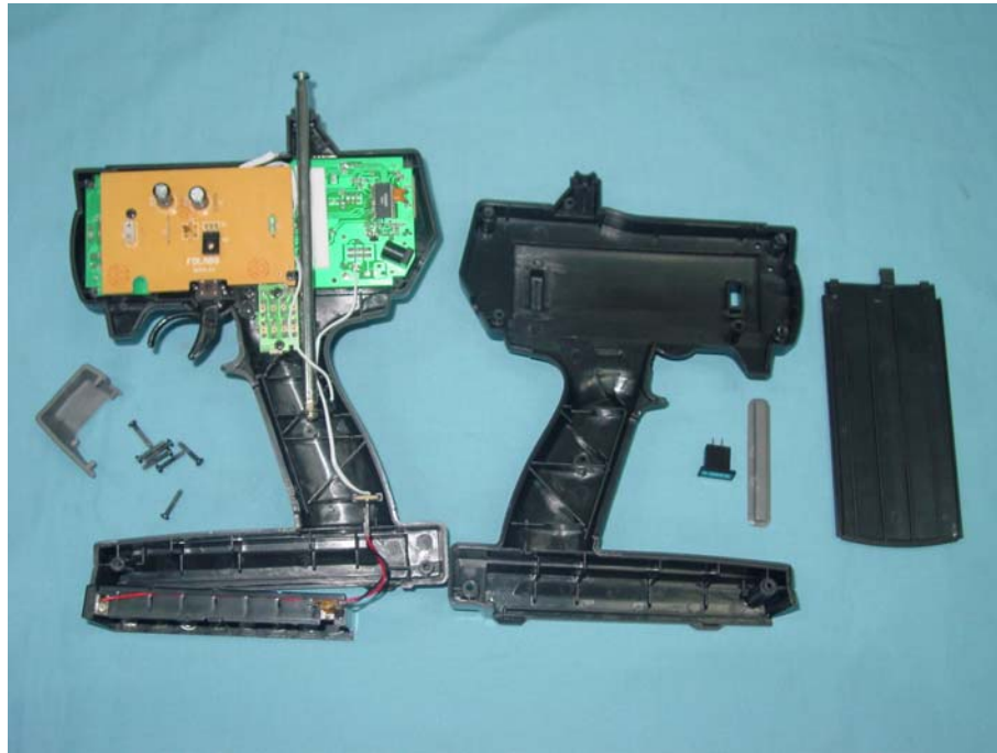
Figure 3 Inside View of the EUT
