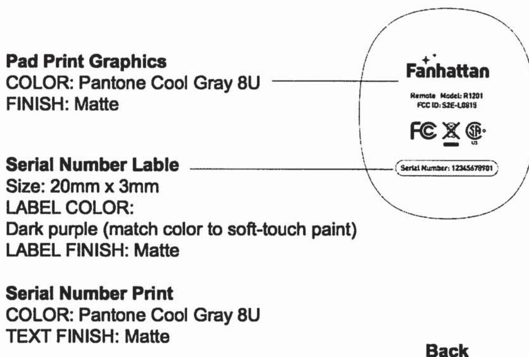
Figure 3: FCC ID S2E-L0815 marking
