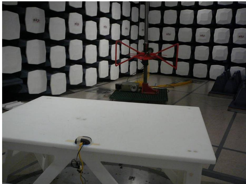
**14.5 Radiated Emission above 1 GHz Rear View at 3 Meter**
