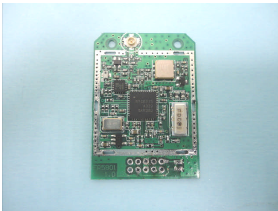
5.8GHz Video receiver module
