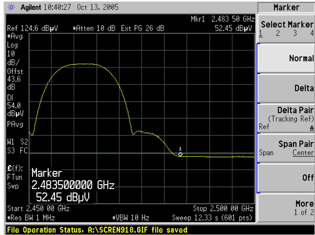
**Band Edges (802.11g / CH Low)****Detector mode: Peak****Polarity: Vertical**
