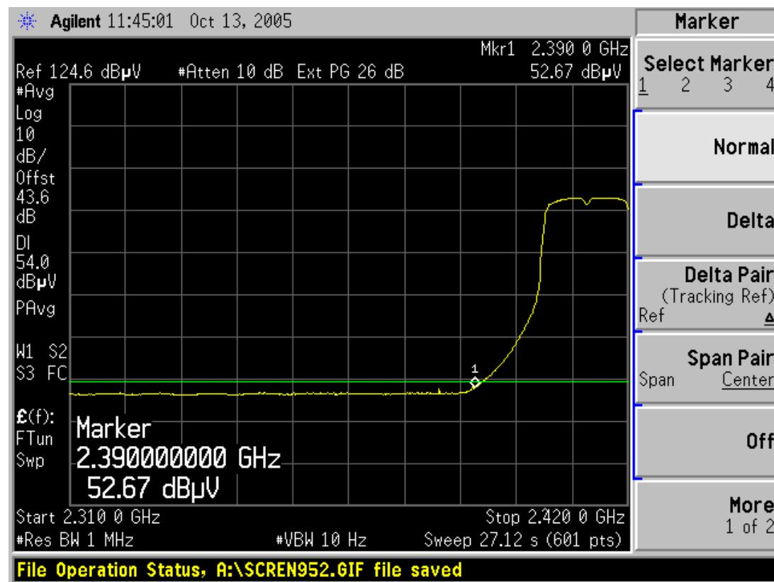
**Band Edges (802.11g / CH High)****Detector mode: Peak****Polarity: Vertical**
