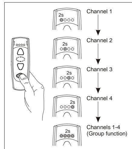
Each time you press the channel selector button, you switch to the next channel or to the group function (channel 1 > channel 2 > channel 3 > channel 4 > channels 1-4/ group function > channel 1 etc.).
