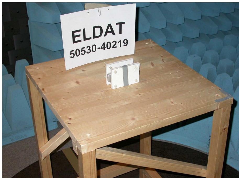
**Test setup for radiated emission measurement
