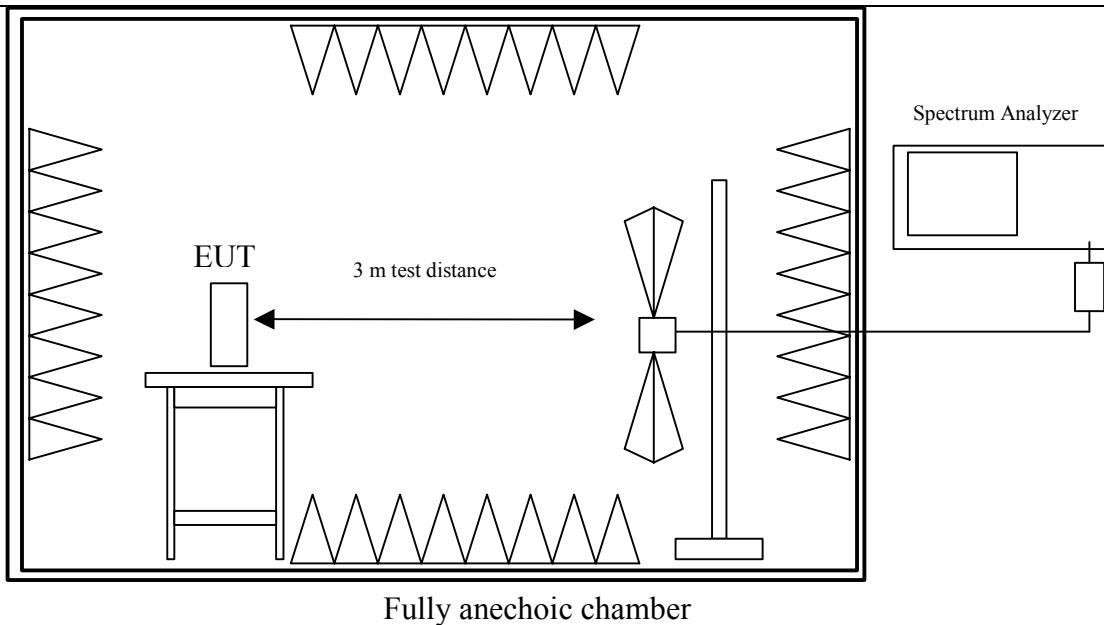
Fully anechoic chamber
