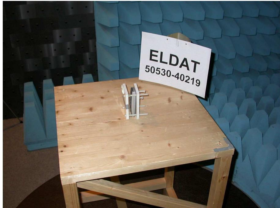
**Test setup for radiated emission measurement
