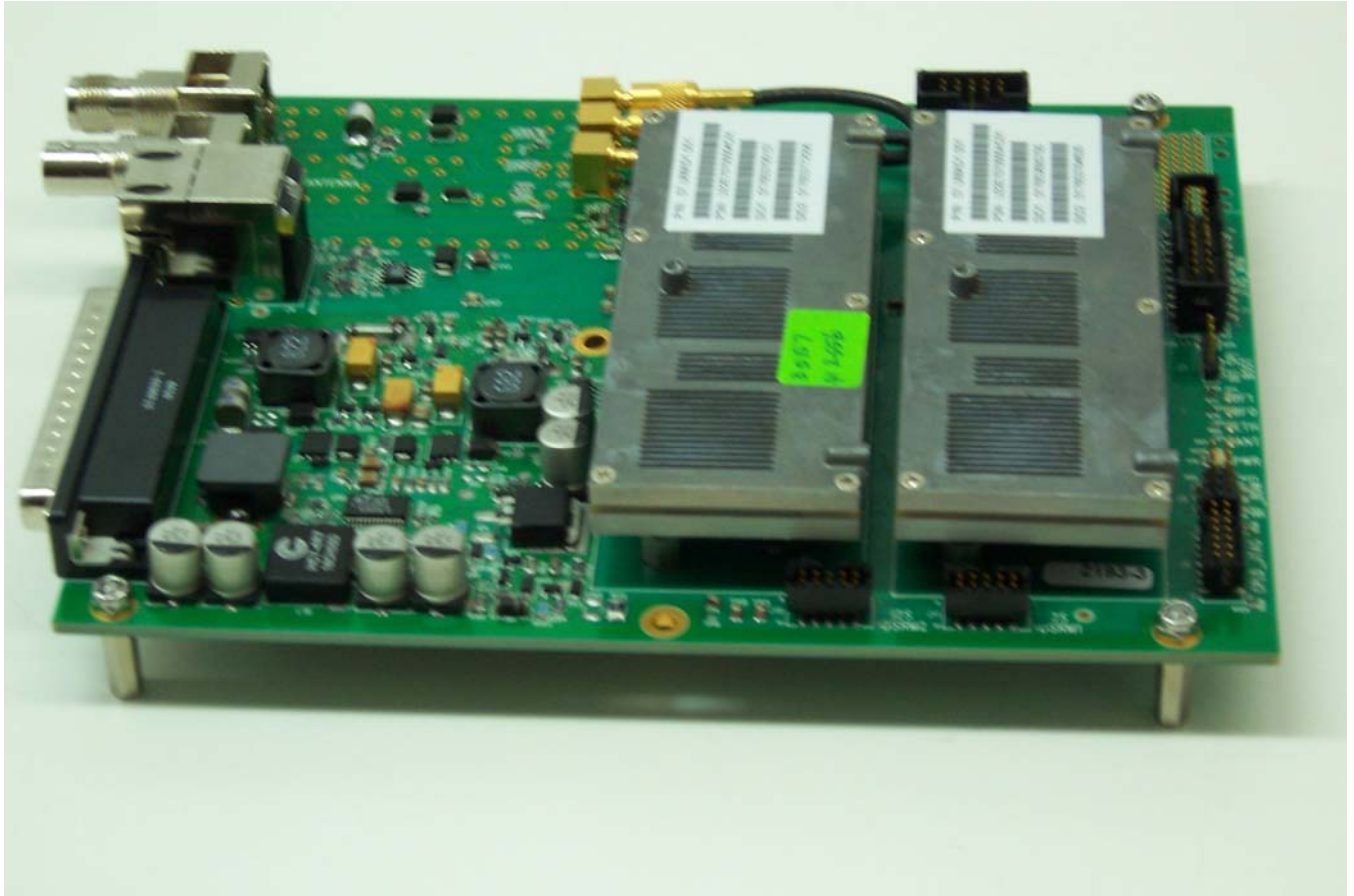
Main PCB with modules installed
