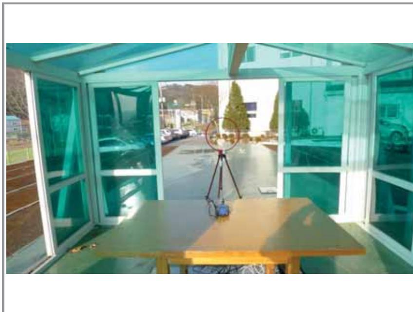
**Photo of radiated spurious emission at 30 MHz ~ 1 000 MHz**
