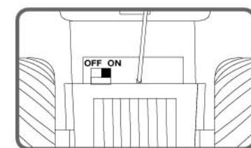
The power switch is located behind the vehicle (as shown). Please make sure it is the ON position when you operate, and OFF position when not in use.
