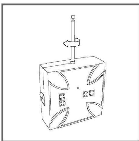
Tighten the antenna into the Transmitter.
