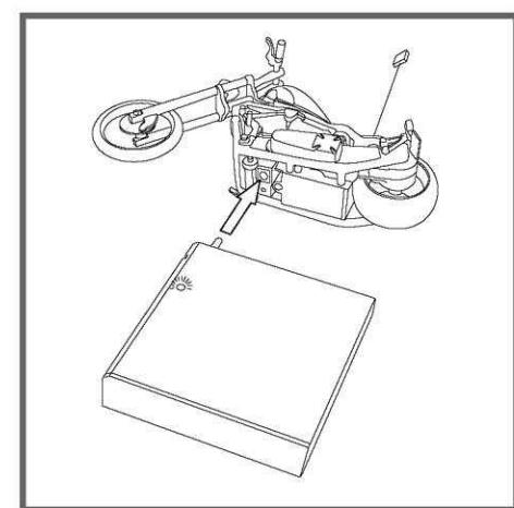
Insert charger pack into socket under the bike wait until the LED indicator turns off (90-120 seconds).
