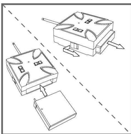
Insert battery pack into the transmitter. Push button to release battery pack.
