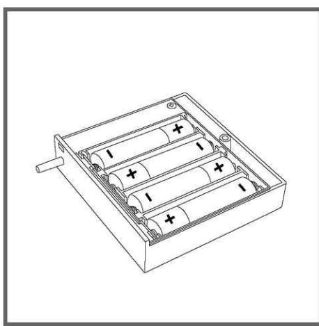
Install 4 AA alkaline batteries with polarity (+/-) as shown inside battery compartment.
