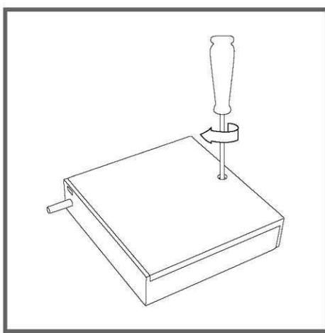
Close battery door and tighten screw.
