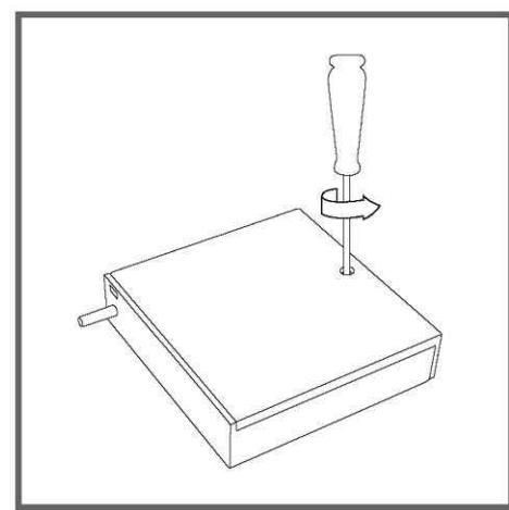
Unscrew battery door with a Philips head screwdriver (not included).
