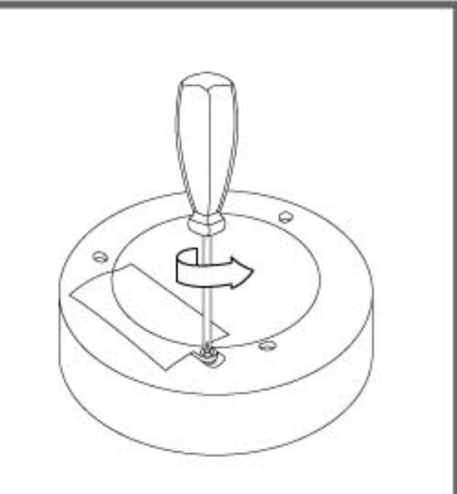
Remove battery door with a Philips head screwdriver (not included).
