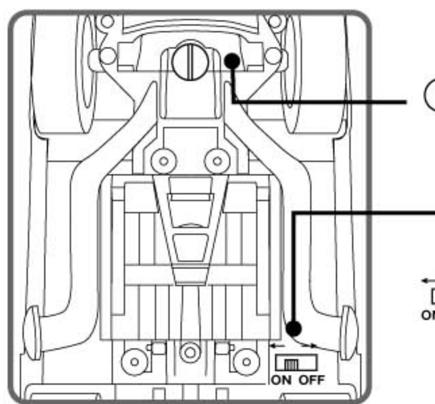
If the car does not run in a straight line, adjust the angle with this lever.
