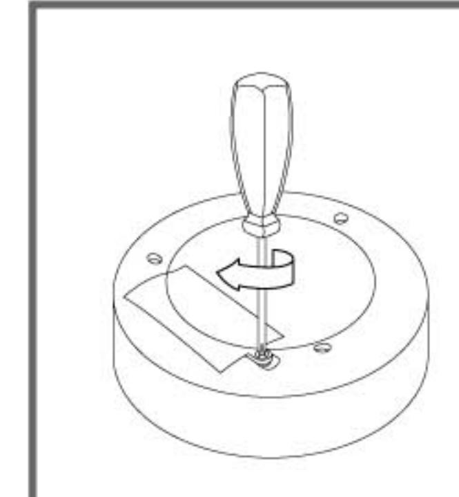
Replace battery door and tighten screw.
