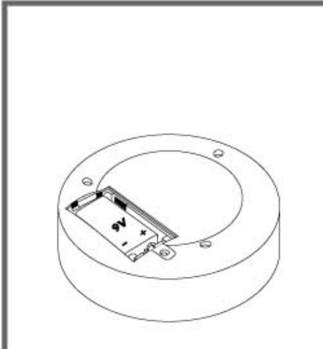
Install one 9V battery with polarity (+/-) as shown inside battery compartment.
