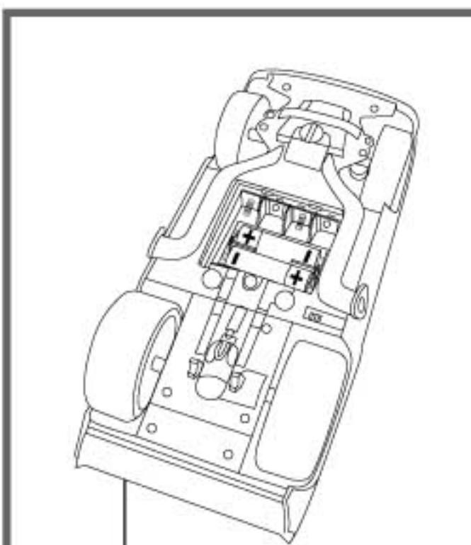
Install 2 AA batteries with polarity (+/-) as shown inside lower battery compartment.
