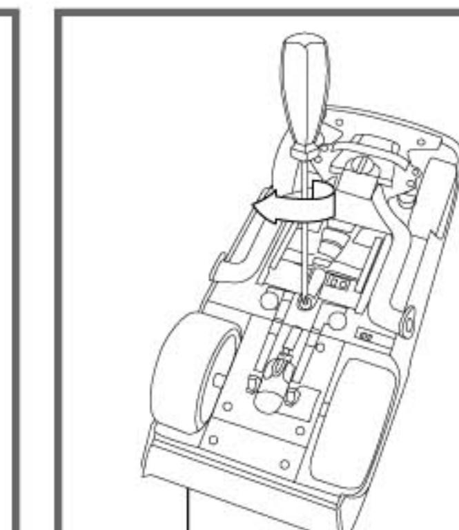
Tighten battery door with a Philips head screwdriver (not included).
