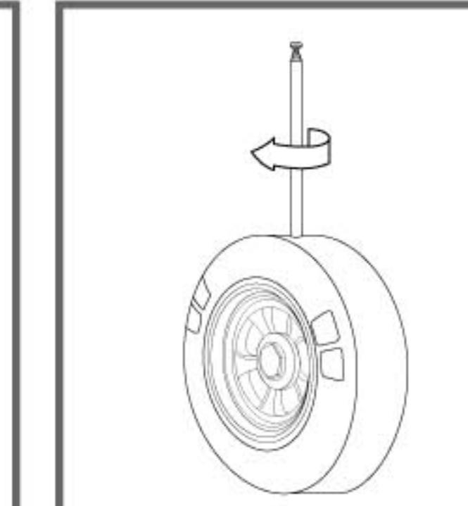
Tighten the antenna into the transmitter.
