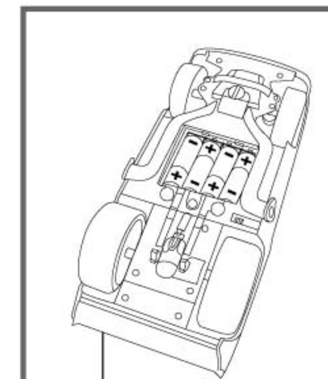
Install 4 AA batteries with polarity (+/-) as shown inside upper battery compartment.
