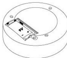
Install one 9V battery with polarity (+/-) as shown inside battery compartment.
