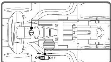
If the car does not run in a straight line, adjust the angle with this lever.
