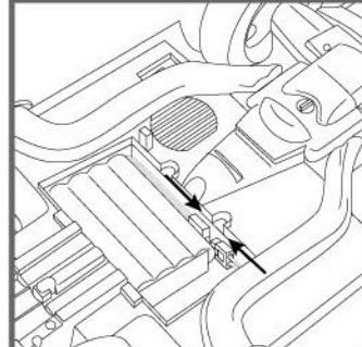
Attach the 9.6V battery pack to the plug inside battery compartment with polarity(+/-). Then place into battery compartment.
