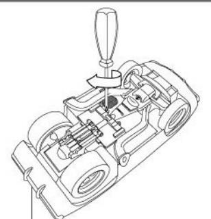
Tighten battery door with a Philips head screwdriver (not included).
