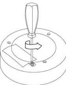
Remove battery door with a Philips head screwdriver (not included).
