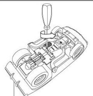
Remove battery door with a Philips head screwdriver (not included).
