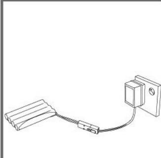
Attach the 9.6V Ni-Cd battery pack to the battery charger, then plug the battery charger into a standard wall outlet.
