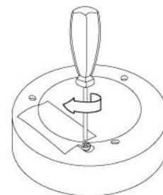
Replace battery door and tighten screw.
