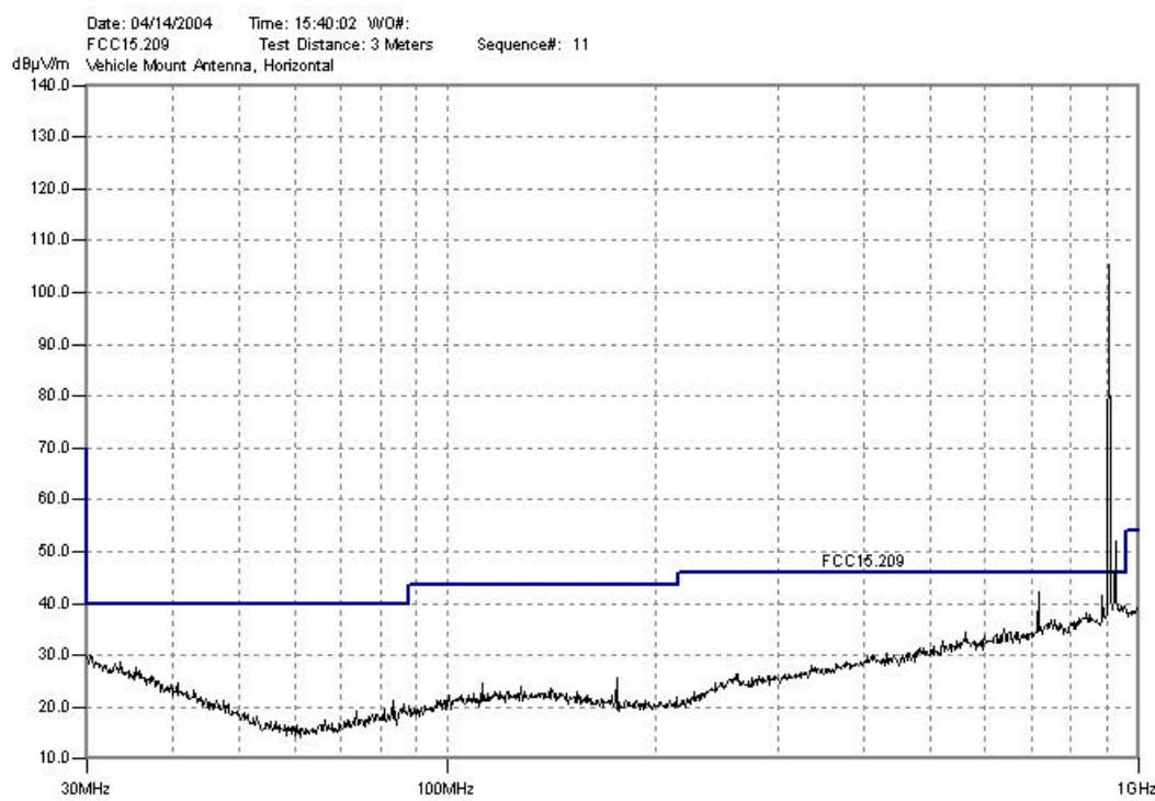
Note: Largest spur around 700MHz is outside a restricted band and only required to be -20dBc.
